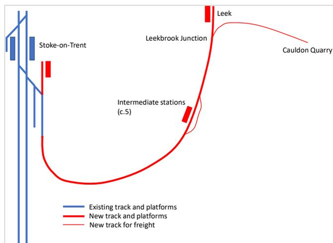
*Figure 18 - Concept track layout for Option B (freight)*
