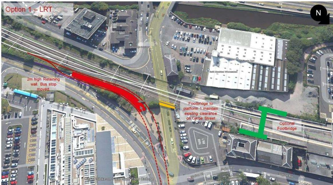
Figure 15 - Potential light rail adaptation to allow street running. Background image Google 2022 ©
